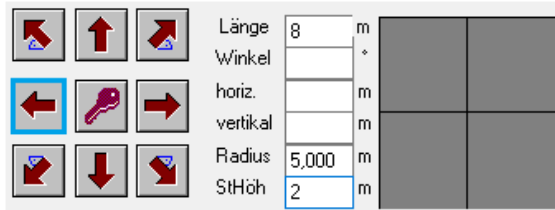
Image 2.5) rounding with a length 8 m and rise 2 m
